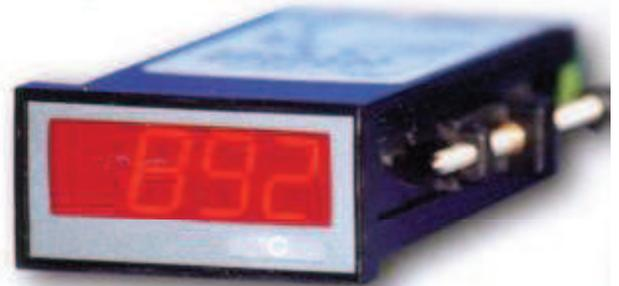
This display unit was developed for use with our high temperature sensors. As it has a circuit onboard it is easy to install. Only four connections have to be linked; 2 for the 12 V DC power supply and 2 for the temperature sensor. There is no need to use the voltage divider VD-200 if the DU-200 is used alternatively.
